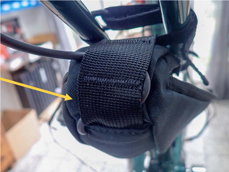
Potentiometer cable S-shaped through the front loops for strain relief
